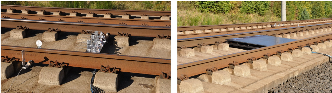
Figure 55: Full-scale measurement set-up: vertical rakes of Pitot-probes together with a light gate for the determination of the air velocity and train speed, respectively (left), and a static surface pressure plate with distributed pressure taps (right).
