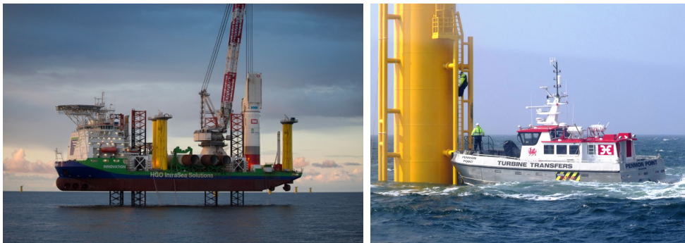
Figure 1.2: Left: Jack-up rig elevated in sea (©Magnus Reinke). Right: boat-landing for safe transfer (Source: Turbine Transfers Ltd).
