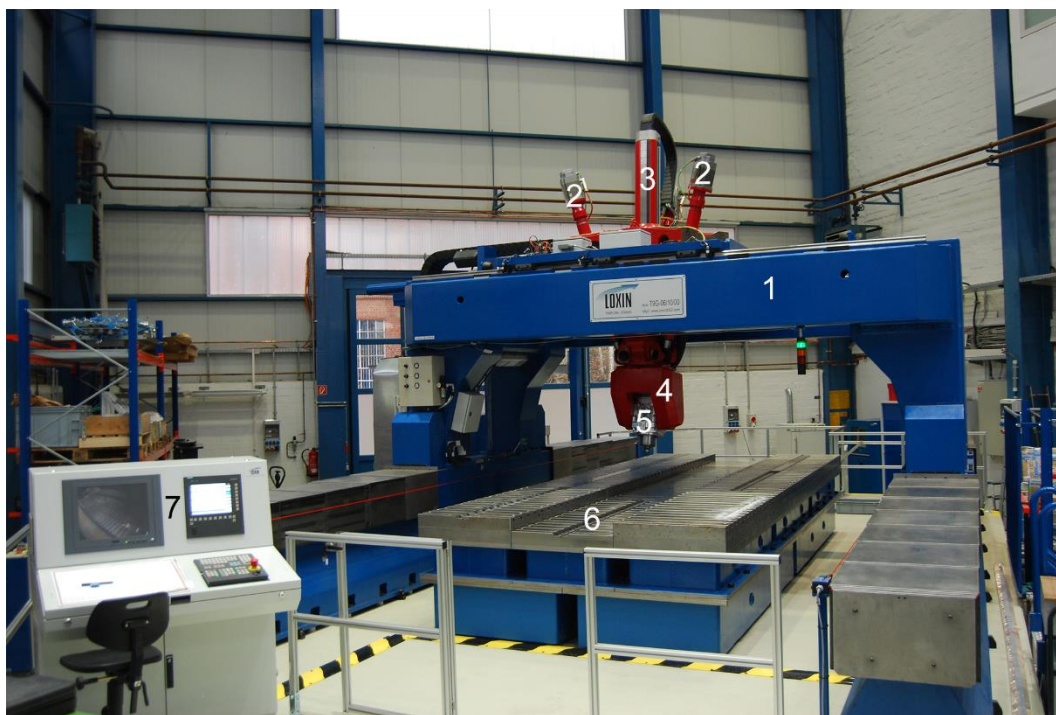
Figure 3.3. Gantry Tricept T9000 welding machine for FSW
