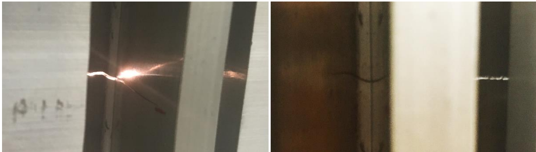
Figure 8.3. Different crack propagation behaviour between the right and the left crack at the skin-stringer weld for the specimen 5-S-4
