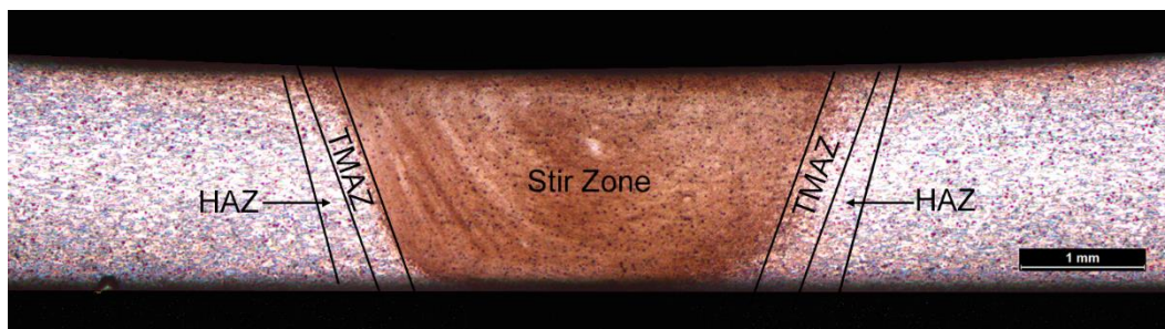
Figure 2.3 Example of SSFSW cross-section with different weld zones
