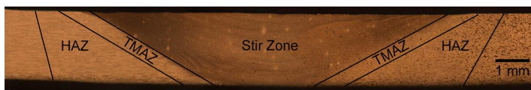
Figure 2.2. Example of an FSW cross-section with different weld zones
