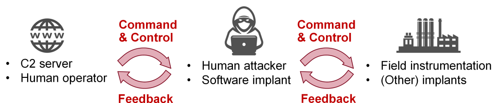
Figure 6.14: Architecture of C2 and feedback channels in cyber-physical attack life cycle
