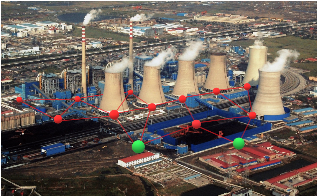
■ Figure 1.1.: Exemplary wireless sensor network for the controlling and monitoring of a power plant. 1
