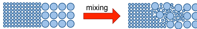
Figure 6.1: Lagrangian variable resolution (fixed masses). Initial (left) and subsequent (right) particle distribution: small particles can penetrate into a large particle region.
