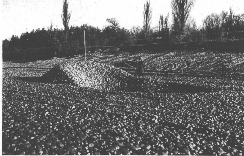
Figure 1.3: Scouring of the waterway bottom induced by an inland vessel during a full-scale experiment by Felkel and Steinweller [24].
