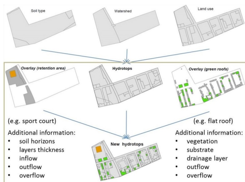
Figure 1. Spatial intersection and aggregation define equal hydrological response units (hydrotops). The new hydrotops contain the SUDS information in the overlay data sets
