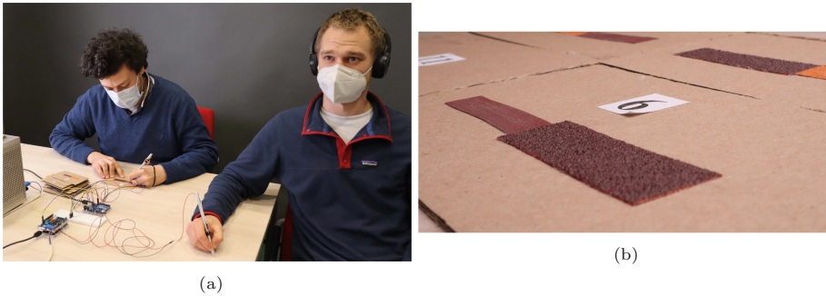
Fig. 1. (a): Case study to judge upon the performance of different vibrotactile actuators. (b): Texture sample. The roughness of second half is higher than the first half.
