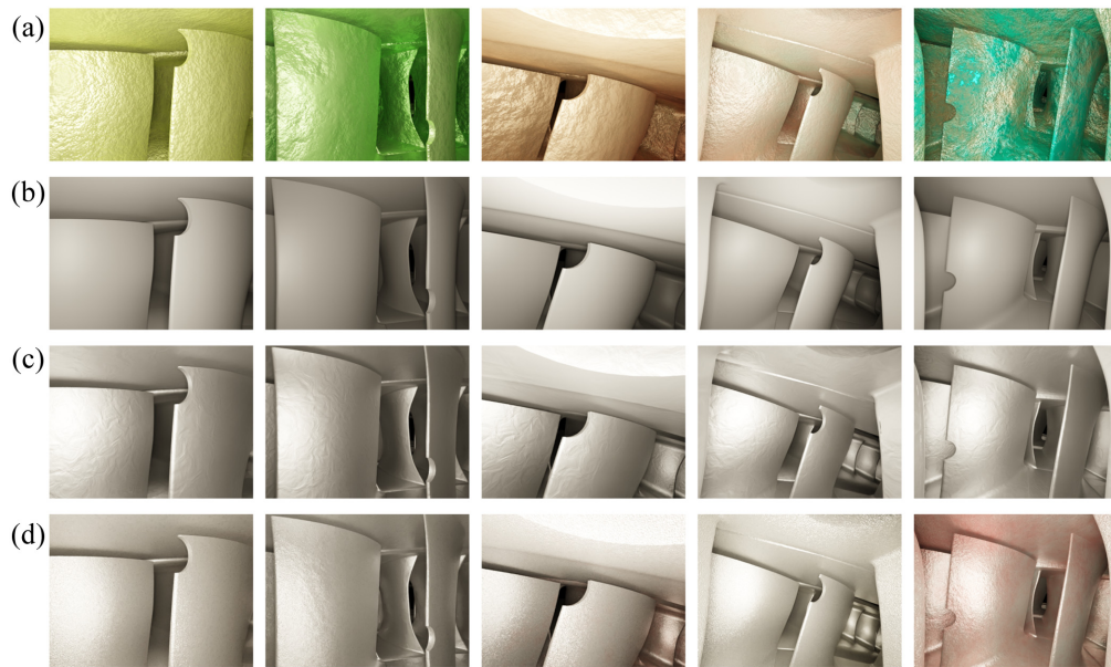
Fig. 8 Samples of synthetic defects with different material models used in the optimization study. (a) Fully randomized. (b) Plain gray. (c) Metal. (d) Randomized metal.
