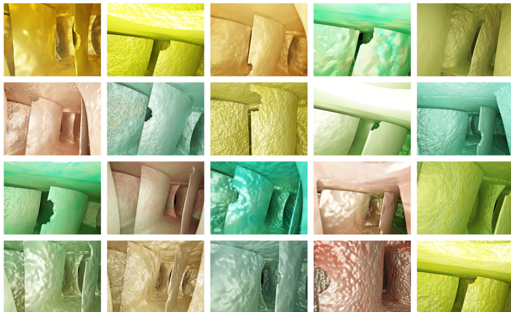
Fig. 9 Representative samples from the best-performing synthetically generated dataset using the developed rendering pipeline. These examples illustrate variations in viewpoint, defect position and shape, and material appearance.
