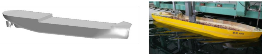
Figure 1: model and numerical TSHD model
