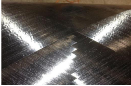
Figure 5-3 \pm 30^\circ Crossing of +30^\circ and -30^\circ tapes
