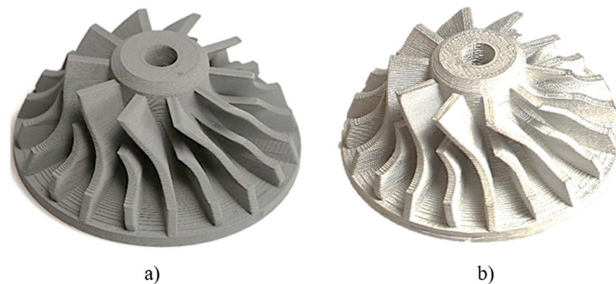
Figure 24. A 316L impeller fabricated using the MEX/M process. (a) The green part is on the left; (b) the sintered part is on the right.
