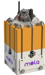
Figure 1: CAD model of the Modular Ocean Lander (MOLA).
