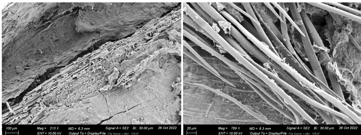
Figure 2: Scanning electron microscope images of BSG fiber structure. Left: 213x magnification of BSG lignocellulosic surface structure. Right: Close-up of 789x magnified cellulose fibrils.
