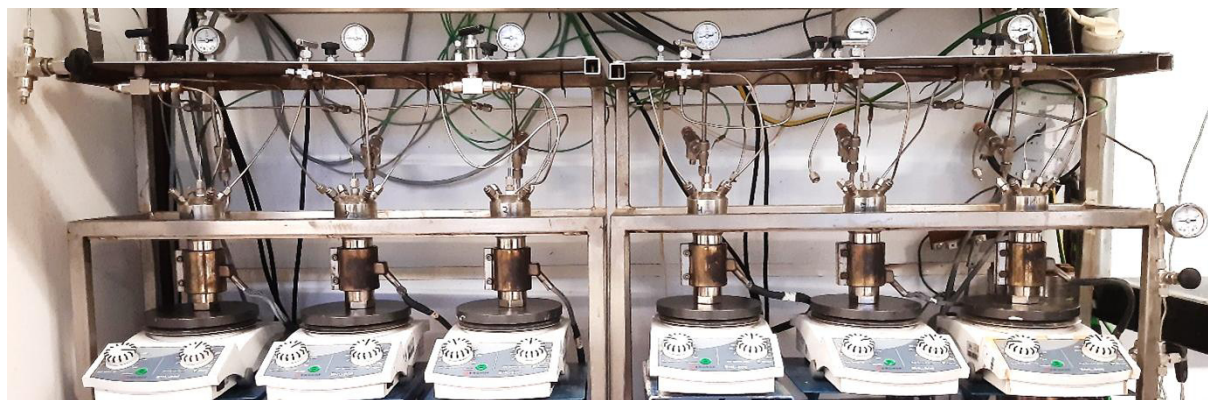
Figure 8: Experimental set-up of 30 mL batch reactors for liquid hot water extractions.
