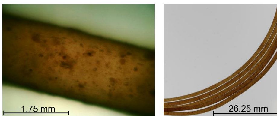
Figure 85: 5% by weight pre-compounded BSG in PLA filament extruded at 195 °C, 5.5 rpm and 65% fan speed. Left: BSG particle distribution in 5x magnification through light microscope. Right: Full view of extruded filament strand.
