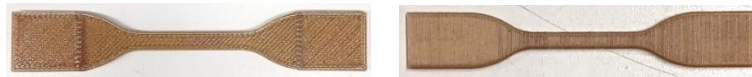
Figure 89: 3D printed test specimen according to ISO 527-2. Left: Printed in x-y direction. Right: Printed in z direction.
