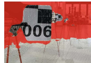
Figure 5: Example out of a static scan experiment, which didn't work to get the length of 5 m, only 2 m. The density of the point cloud was too low, experiment (iii).
