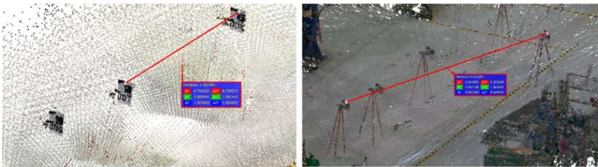
Figure 4: Process of the manual measuring in the point clouds, between the used target markets in experiment (iii), to get the length between target markets in the Software CloudCompare. From left to Right side: Scaniverse, BLK2GO.
