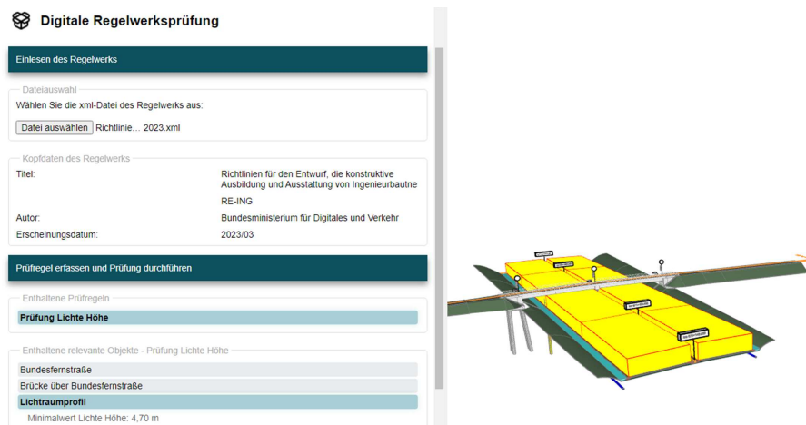
Figure 2: Developed Desite BIM Plugin and the tested BIM Model
