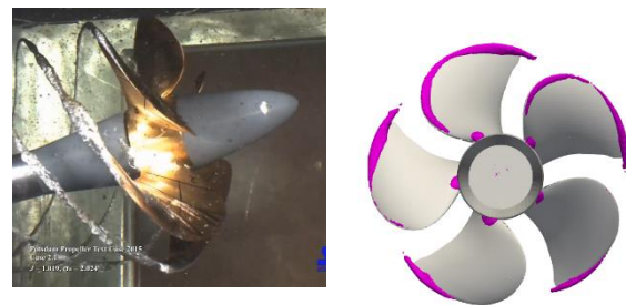
Figure 6 Comparison cavitation observations (SVA Potsdam, 2015) vs. interpolated FVM prediction
