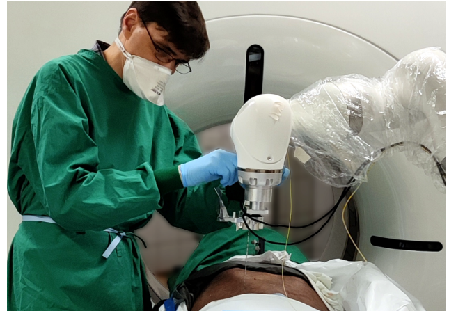
Fig. 1. Collaborative Robotic Biopsy: The robot guides the needle trajectory while the physician inserts the needle. Needle tip forces are sensed by the physician through haptic feedback allowing him to feel tissue interfaces during the needle insertion.
