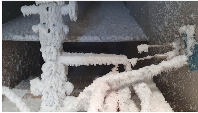
Fig. 4. Frozen humidity on the DCB specimen during low temperature testing.
