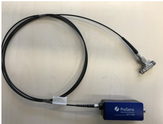
Figure 3-4: Measuring system FTM-Pst3 and processing unit OXY1-SMA
