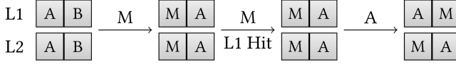
(a) Simulation of the access sequence M, M, A. The second access to M and the access to A result in an L1 hit.
