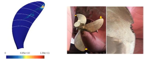
(b) Comparison between numerical cavitation erosion risk results and experimental results for Case 2
