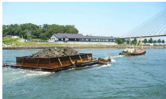
Figure 1: Soil pontoon using knockdown pontoon
