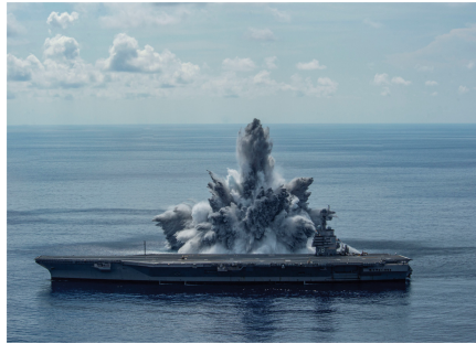
Fig. 18. FSST Test for Aircraft carrier USS Gerald R. Ford (2021)
