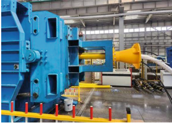
Fig. 14. End termination strength test of 66 kV power and hydraulic combined umbilical.
