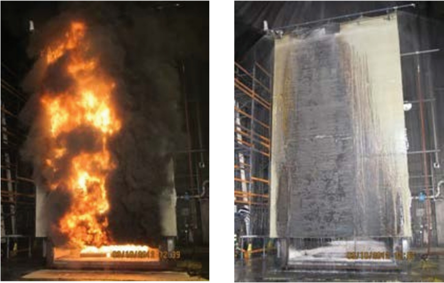
Fig. 11. Fire resistance test of load bearing FRP composite bulkhead with design loads
