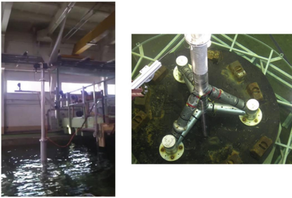
Fig. 20. The wind turbine model with FBG sensors fixed to the partially submerged (Min et al., 2021)
