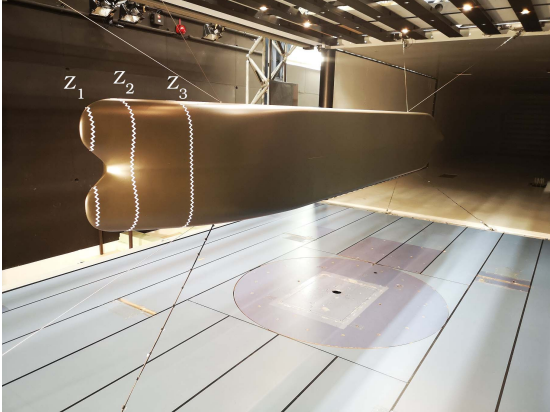
Figure 3: JBC double hull mounted on motion simulator in the low speed wind tunnel of TUHH
