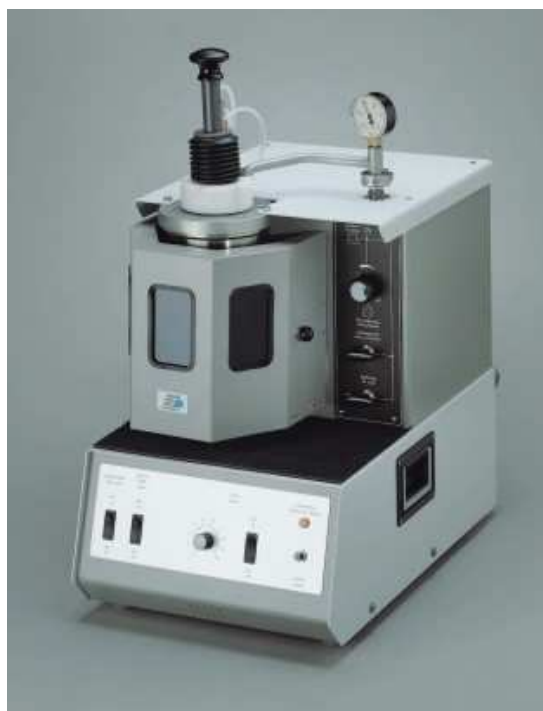
Figure 3.2: Mini arc melter used to prepare alloys in present thesis.
