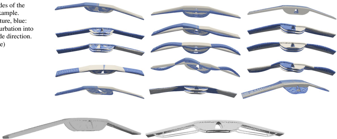
Fig. 14 Final designs of the optimizations of the 3D shallow arc example. Left: Deterministic optimized, right: robust optimized
