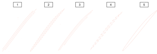
Figure 6: different path planning strategies for build-up welding using the example of a sheet cut/layer
