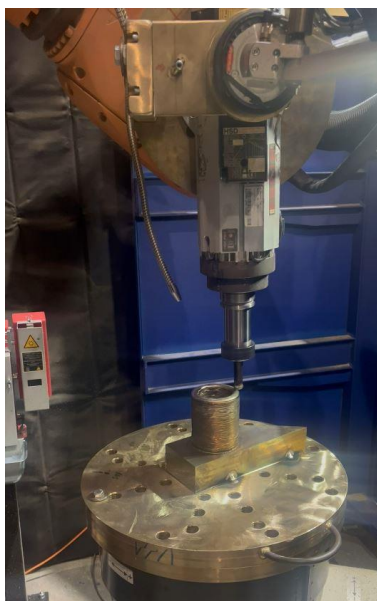
Figure 7: Indexable insert milling cutter for mechanical machining to correct the layer height
