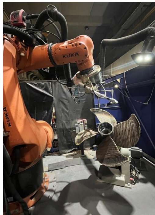
Figure 8: propeller as-fabricated state by additive manufacturing
