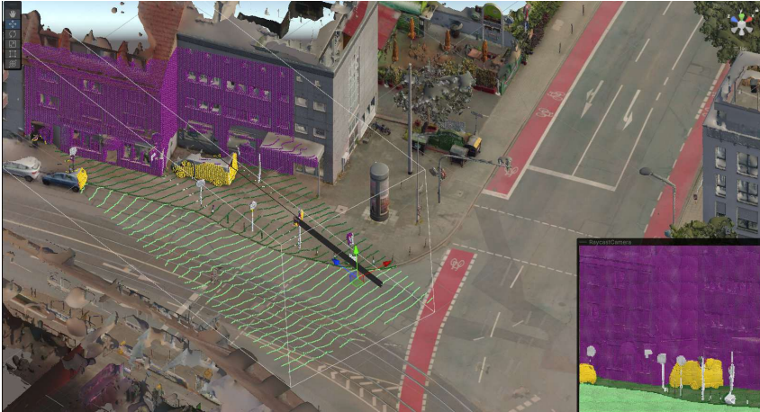
Figure 4: Visualisation of the segmentation results with lines and spheres as 3D representation of the raycast hits.
