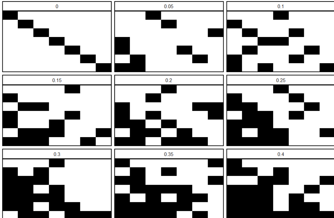
Figure 3.12: Patterns created using EAD's domain mapping matrix procedure. The numbers on top of the subplots represent the normalized system design complexity ( SDC_N ).
