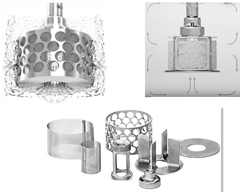
Figure 2. The rotating bed basket from SpinChem AB. The predicted flow pattern (top, left) around a SpinChem® rotating bed reactor S2 in vessel V2, simulated using Ansys Fluent, SpinChem AB [44]. The inside of the rotating bed basket was filled with solid particles (top, right, SpinChem AB [45]). The elements of the rotating packed bed reactor S2 assembled to form a basket with a stainless steel (SS316L, EN2348) filter inside (down, SpinChem AB [46]).
