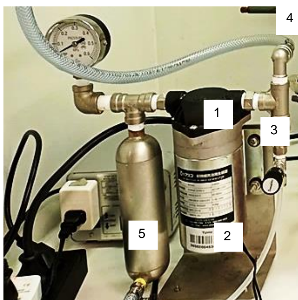
Figure 8. AMB3 fine bubble generator: 1 - mixing vessel: air with water, 2 - air suction, 3 - air control valve, 4 – liquid inlet, 5 – liquid discharge with fine bubbles [84].
