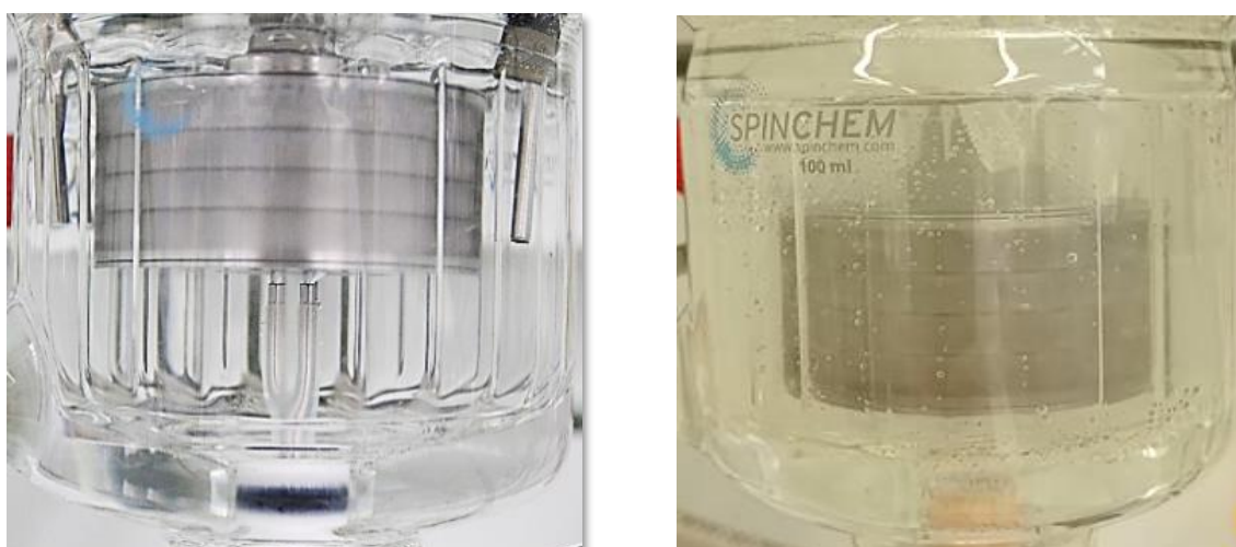
Figure 21. The SpinChem® vessel V2 equipped with two different aerators. Aeration by the open tube sparger (orifice diameter: 2 \text{ mm} ) with macrobubbles (left), milky with fine bubbles generated (right) by the AMB3 fine bubble generator.
