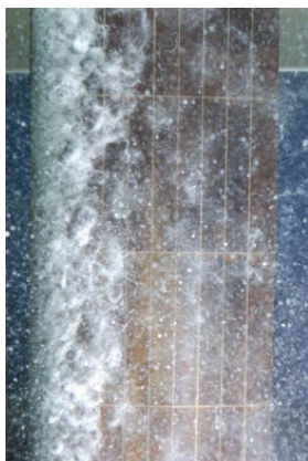
Figure 5.10: Sheet cavitation extent measured in experiment for the simulation case 2 and \sigma = 3.0 with air content of 80% (taken from Richter (2011, p. 4.10))
