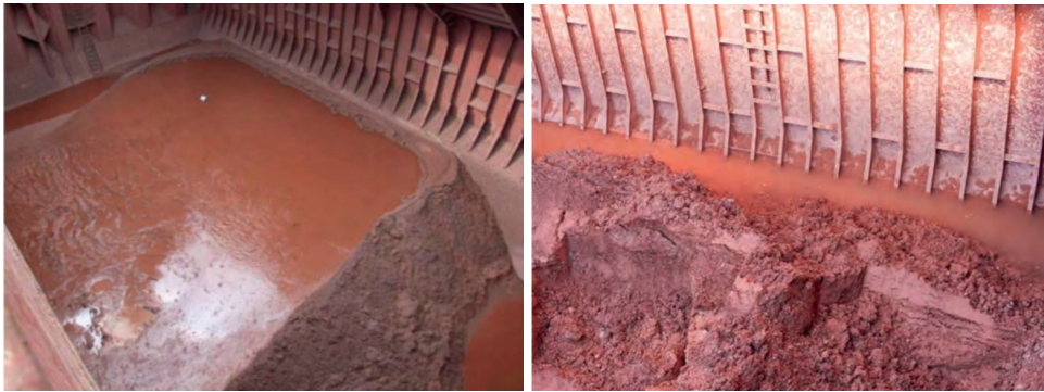
Figure 1.4: Bauxite cargo exhibiting water separation on the top of the cargo pile and in the corners of the hold. Extracted from the report of the "Global Bauxite Working Group" (GBWG) [41].
