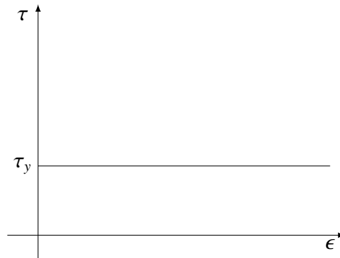
Figure 3.1: Stress-strain relationship of rigid-perfectly plastic material.
