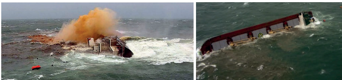
Figure 1.1: Capsizing of bulk carrier "Trans Summer" carrying nickel ore. Photo courtesy to HKG Flying Service, extracted from DNV GL [24] and Munro et. al [89].
