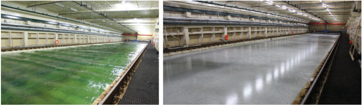
Figure 65: Waves in the basin during WCP (left) and resulting ice sheet ready for testing (right).
