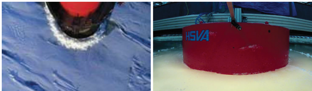
Figure 64: Left: Crushing of sea ice against NSG lighthouse [42], right: crushing of model ice against a cylindrical structure with similar aspect ratio
