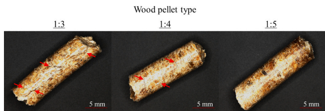
Fig. 4. Optical profilometer images of the surface texture of untreated wood pellets 1:3, 1:4 and 1:5 with surface cracks shown by red arrows. (For interpretation of the references to color in this figure legend, the reader is referred to the web version of this article.)
