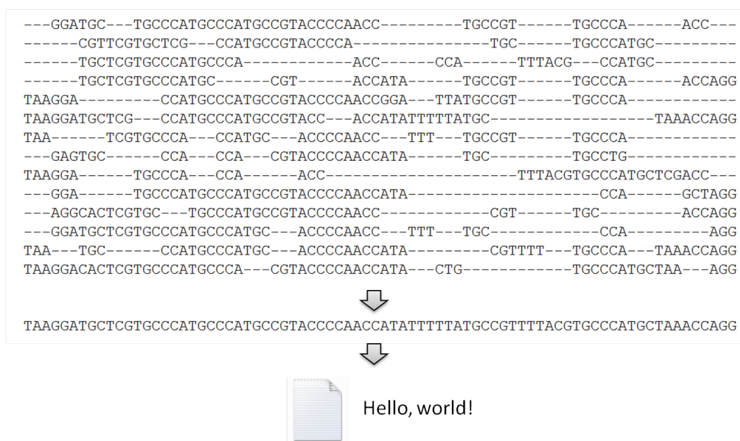
Fig. 5.8 Correct information can be retrieved using 14 sequences with high rates of errors introduced by error-prone PCR.
