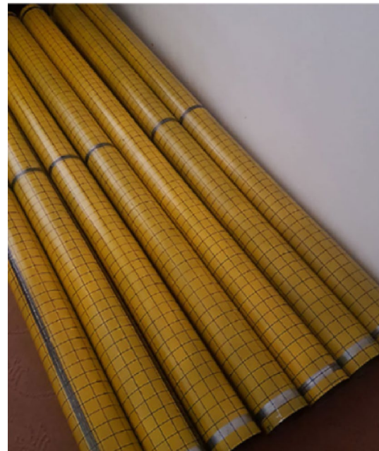
Fig. 5 Mesh drawn lines on the pipe [11]
