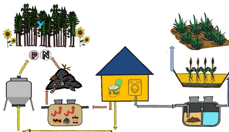
Figure 3 Recommended Integrated Decentralised Rural Wastewater Treatment System
