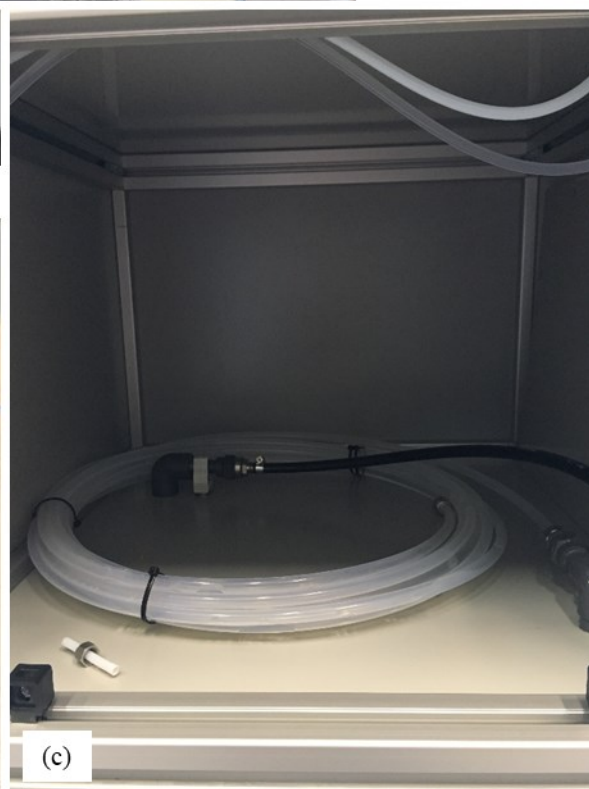
Figure II-9. (a) Small-scale ozonation pilot plant (without biofilters), (b) detail pumping unit (before equipment with additional measuring devices and dosing points), (c) detail reaction tube
