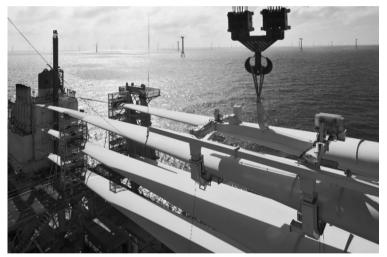
Figure 6: Transport frame for turbine blades on a heavy-lift vessel (Image: Senvion)
