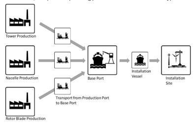
Figure 1: Conventional installation concept (Oelker, et al., 2017)
